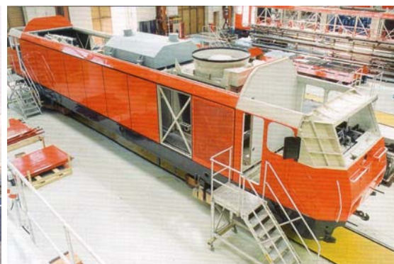
Figure 9.31: An illustration of how the exhaust gas system is accommodated
