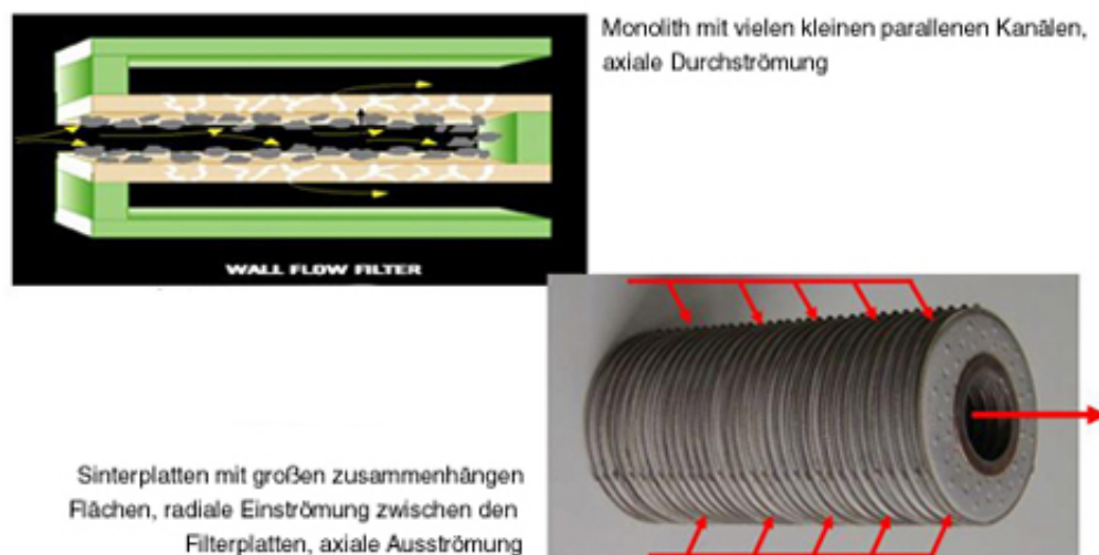
Figure 9.1: Designs of filters for reducing particulates
