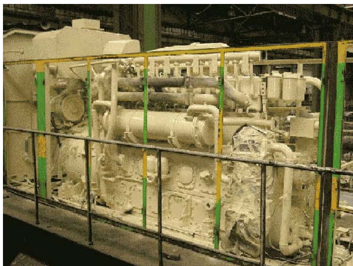
Figure 9.41: Locomotive configuration with engine and exhaust gas unit
