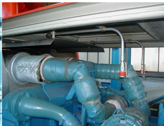
Figure 9.45: Engine-silencer connection on the Class 290 vehicle
