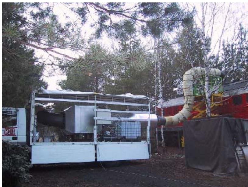
Figure 9.32: Basic tests on a Class 233 locomotive fitted with the SCR system to reduce nitrogen oxides
