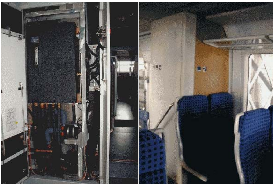
Figure 9.23: Control cabinet with exhaust silencer in the VT 642 passenger accommodation area
