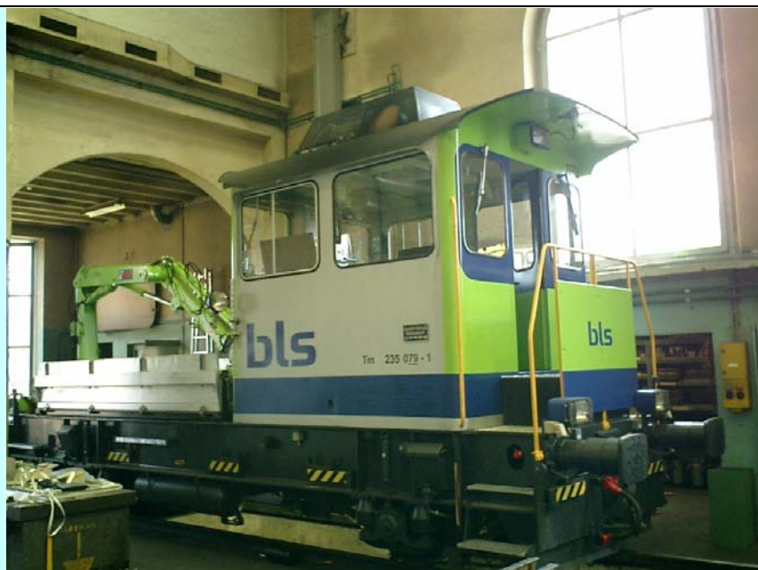
Figure 1. BLS track maintenance diesel locomotive with retrofit DPF (roof of vehicle).
