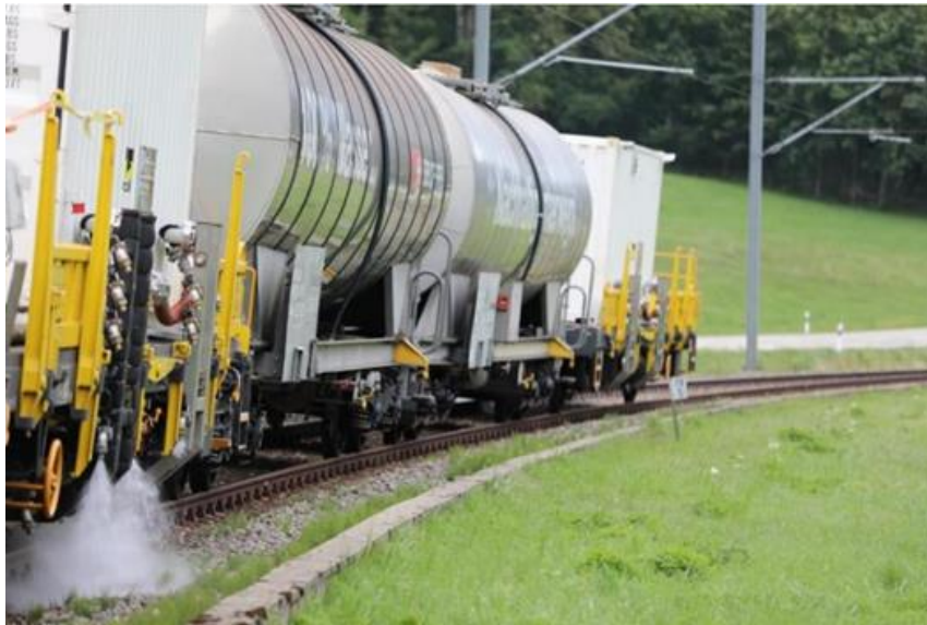
Figure 6: SBB - Hot water spot-spray train prototype
