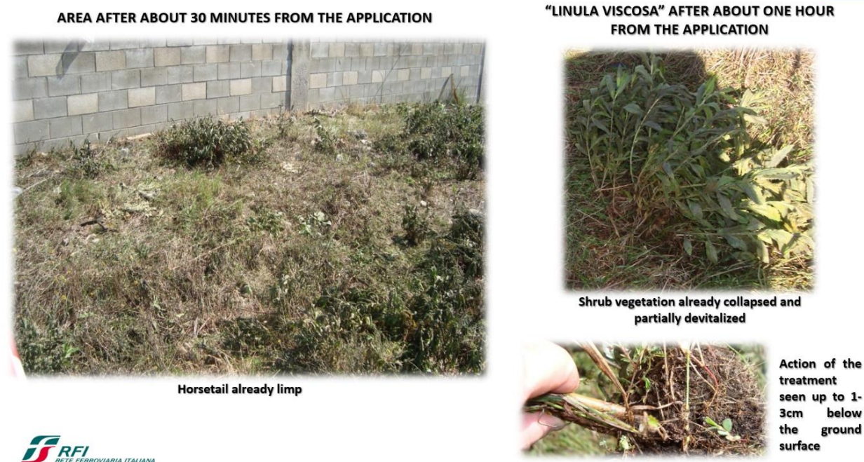
Figure 31: RFI - Hot Foam Method-1 - (a) demonstration test, (b) first results after 30 minutes
