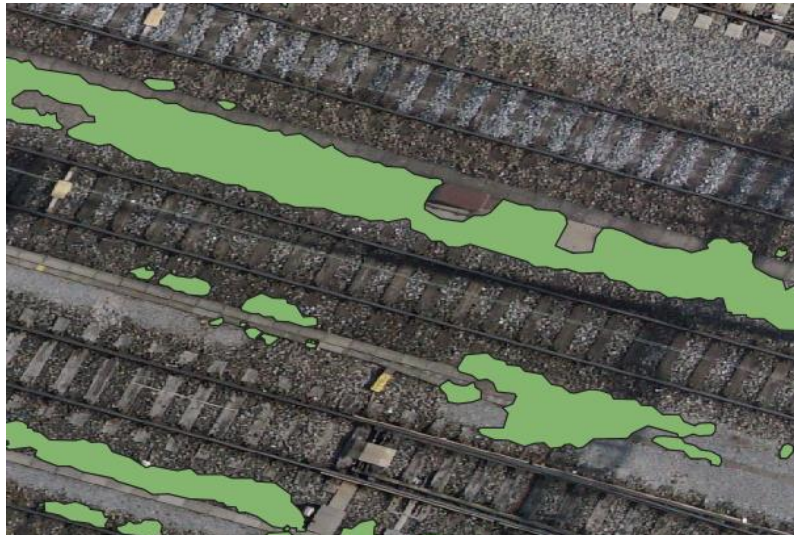
Figure 19: Mapping vegetation with artificial intelligence based on high-resolution orthographic images (example SBB)
