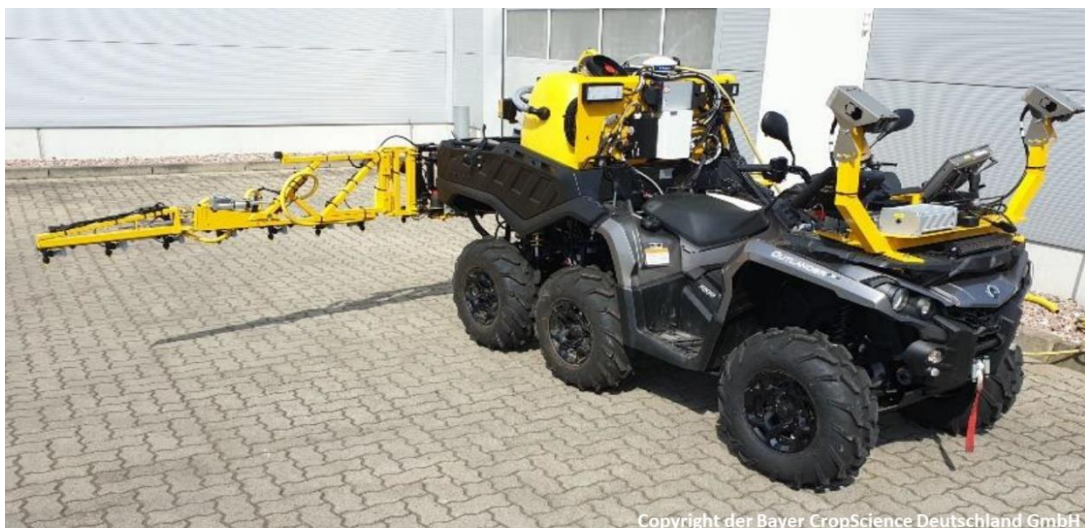
Figure 16: ATV equipped with vegetation detection system
