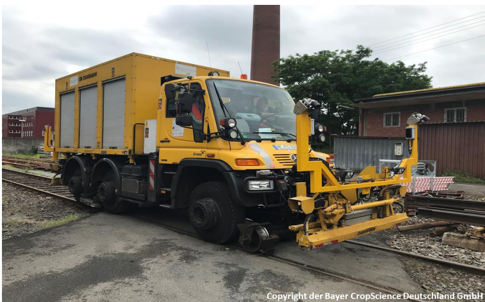
Figure 3: Road-rail vehicle equipped with vegetation detection
