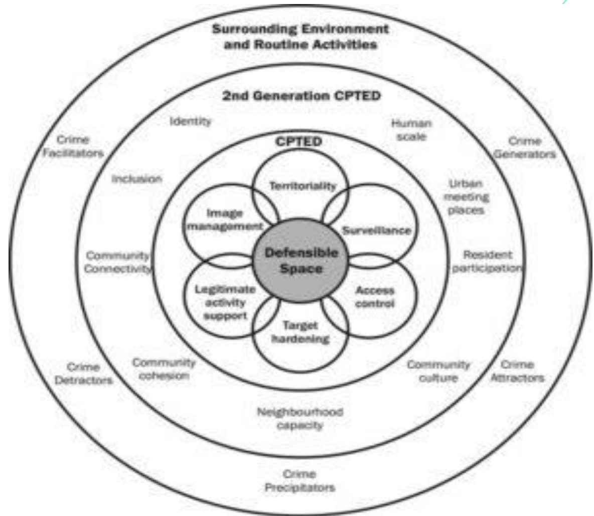
CPTED, second generation dynamic integrated model (Source: Paul Cozens, 2015; adapted from Cozens, 2014)
