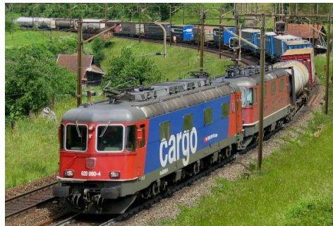
Figure 2: GZ: Freight Train with Re620 Locomotive
