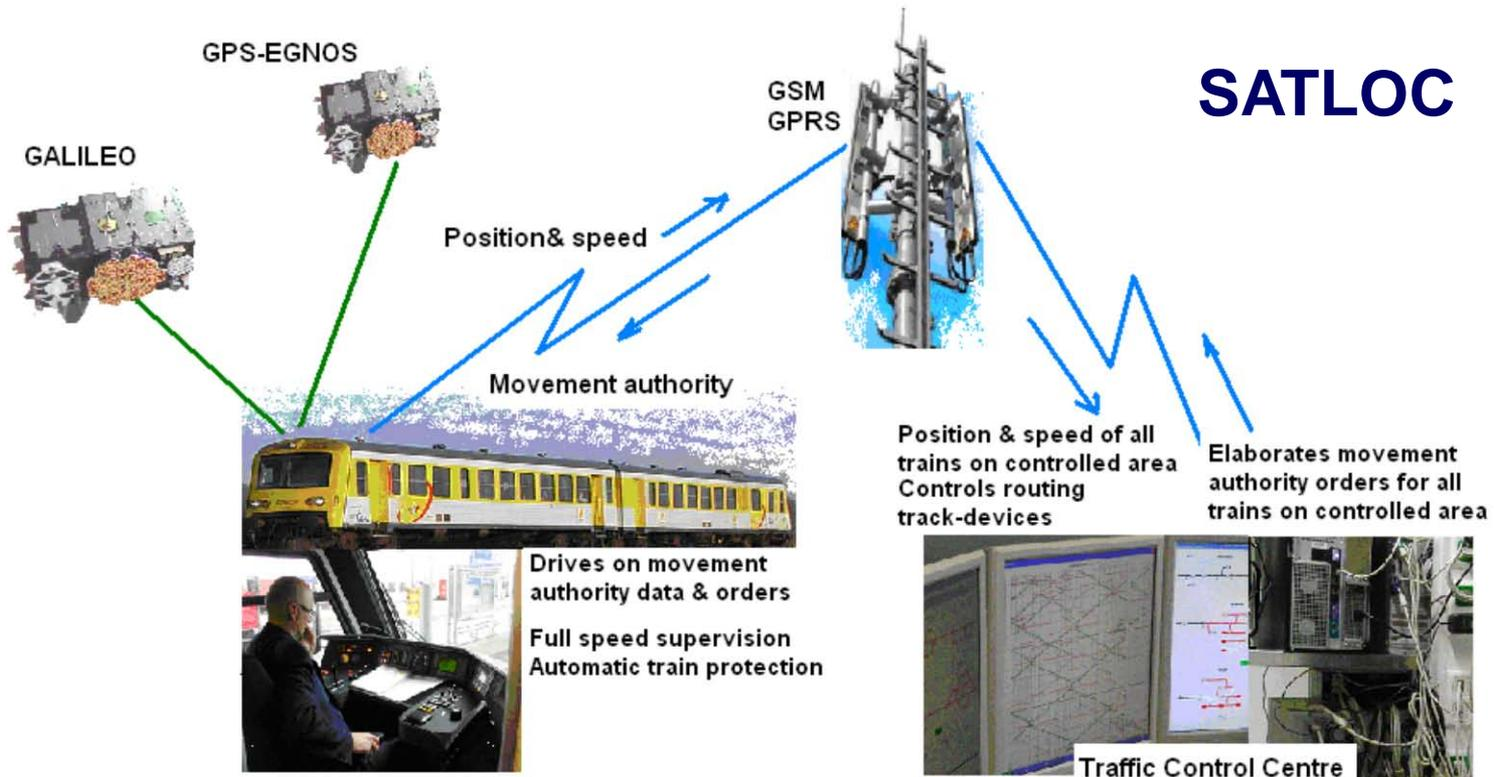
**Principle of satellite & radio-controlled train operation for safety and efficiency on low traffic secondary lines which are not submitted to the EC interoperability by ETCS**
